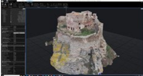
Fig. 11- Photogrammetric processing in EG Reality Capture (graphic elaboration by the authors, 2024).
