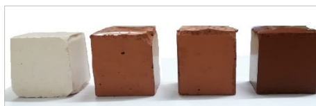
Fig. 2 - Geopolymer samples with different RM amount.
