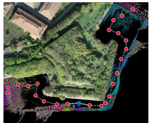
Fig. 8- The 3D scanning network.
