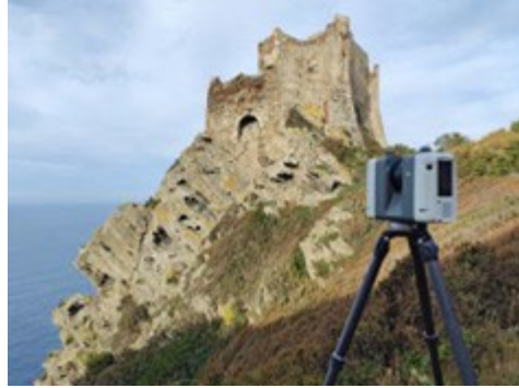
Fig. 6- The Leica RTC360 unit at work during the survey of the Old Tower (photo by the authors, 2024).
