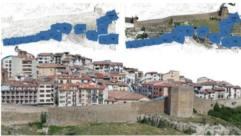
Fig. 3- Acquisition and photogrammetric processing of the city's perimeter defence system. Graphic elaboration by Francesca Picchio, Francesca Galasso, 2024.
