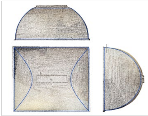
Fig. 6- Vault family laid over the point cloud (graphic elaboration by the authors, 2024).
